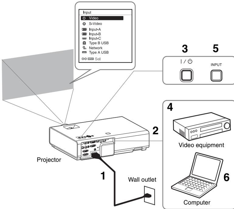
**1** Plug the AC power cord into the wall outlet.
