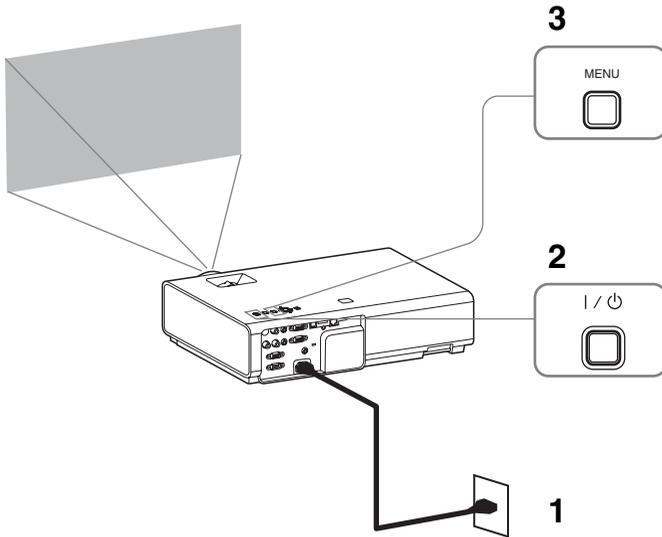
**1** Plug in the AC power cord into a wall outlet.
